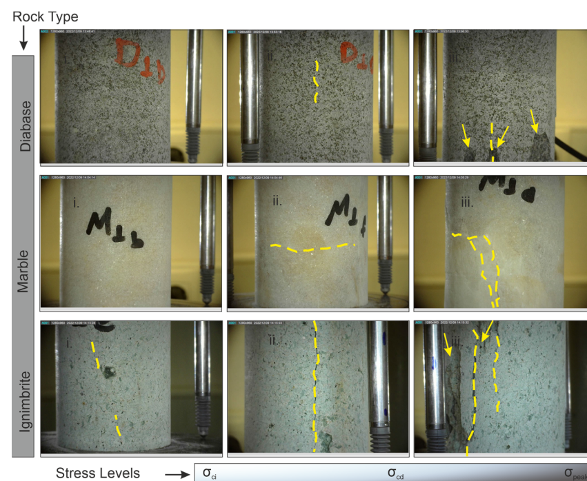
Figure 4. Incremental cracking (mesoscale) with increasing stress under uniaxial compressive loading (i: \sigma_{ci} , ii: \sigma_{cd} , iii: \sigma_{peak} stress levels, and yellow lines: mesoscale cracks).
