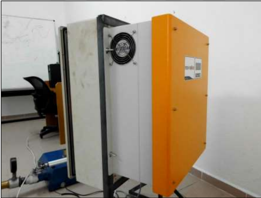
Őekil 4.7 Mavisis marka on-grid Őebekeye paralel inverter
